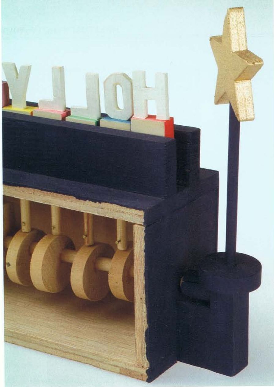
Detail of the friction block into which the friction rod is inserted. The friction collet on the end of the camshaft spins the friction disc when turned.
