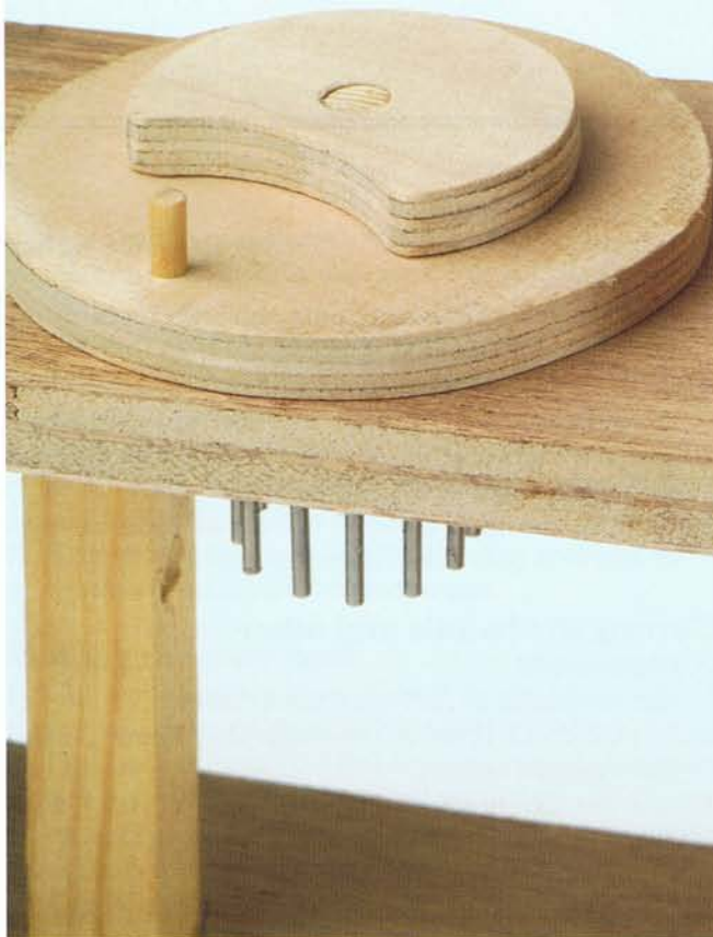
A detail shows a part of the Geneva mechanism, without the cross. Part of the pin wheel attached to the central arbor can be seen with the bearing in the support post on the left.
