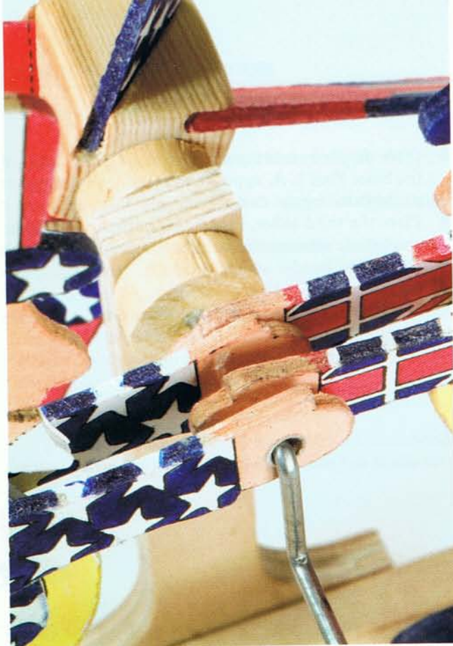
Detail showing disposition of the interleaved hands on the crankshaft. The paddle block is shown with two collets either side of the bearing support.
