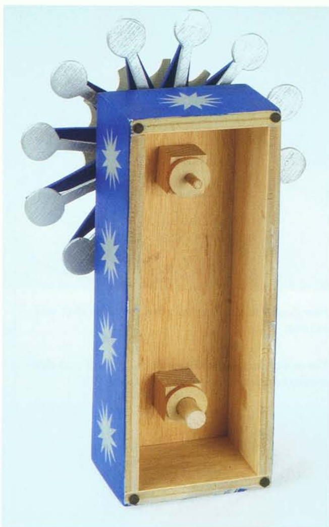
Inside the box you can see the upper and lower bearing extensions and the collet stops.
