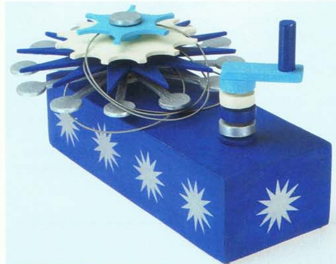
The driving belts, ready to be fixed to the drive shaft, will be twisted to provide backward rotation and placed straight to go forwards.
