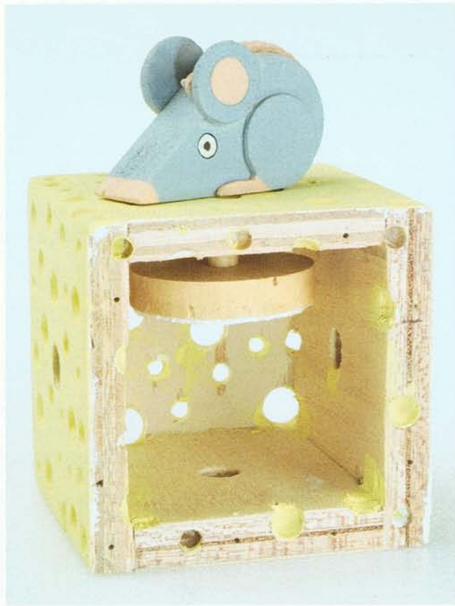
The follower rod is glued into the mouse and inserted through the top panel into the follower disc below.
