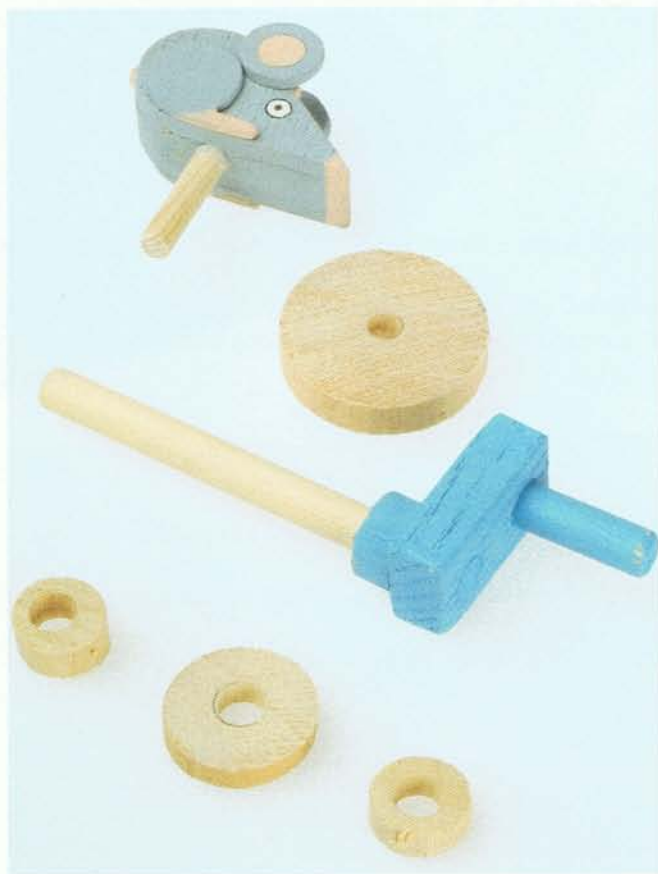
The camshaft handle with the follower disc, mouse and follower rod above the concentric cam flanked by two collets.
