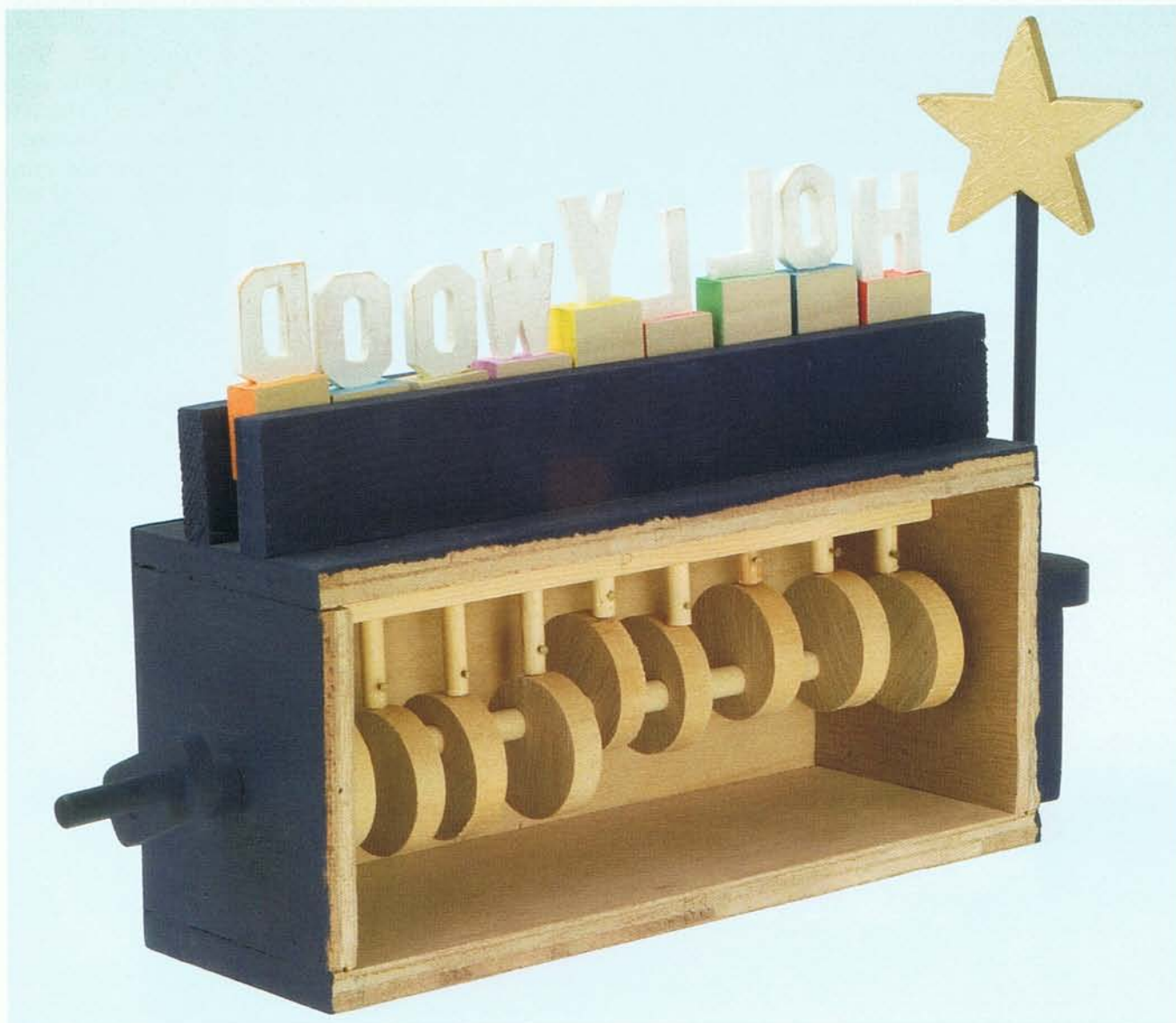
The back panel is removed to show the assembly of eccentric cams' profiles supporting the follower rods attached to the letter blocks.
