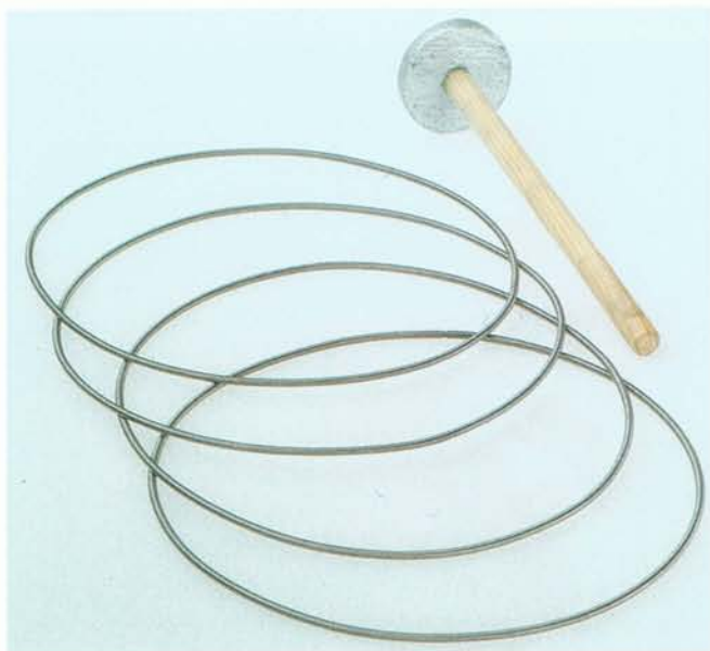
Four flexible steel driving belts and the pulley shaft with end stop.
