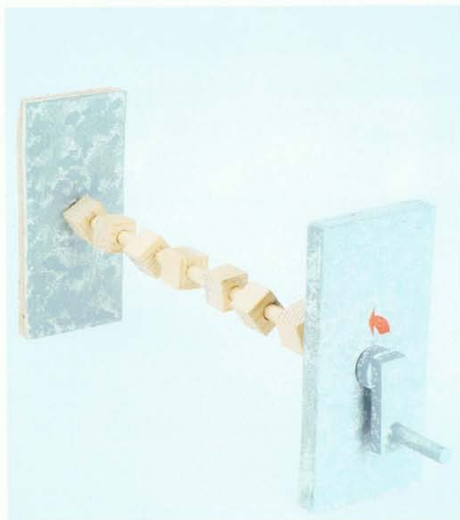
Camshaft held within its side panel bearings.
