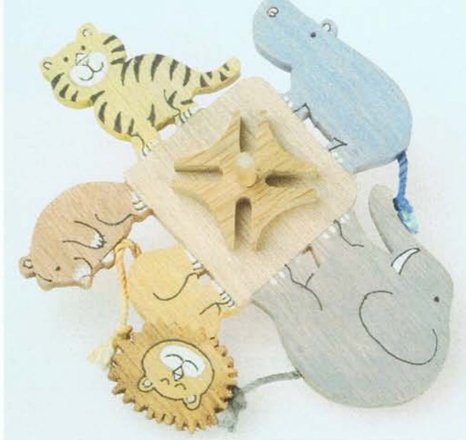
The animals' rotary disc shows the animals, with tails attached, cut from one piece of plywood. The cross on the disc completes the Geneva wheel mechanism.
