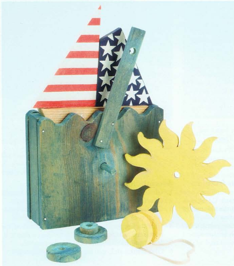
Rear view showing the support bar for the sun glued in position. The two pulley wheels are shown: one complete with pulley shaft, the other open to show the pulley collet. The last stage is to fix the sun and the drive band.
