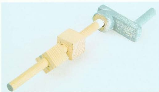
Camshaft with handle and collet and two cam blocks.
