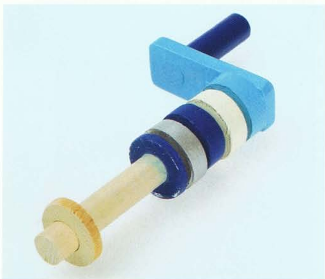
Crank handle and drive shaft with four collets and end stop. The unpainted end stop is fixed to the shaft inside the box.
